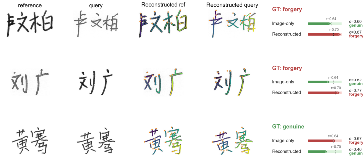
Fig. 4: Qualitative examples showing how reconstructed trajectory guidance improves offline signature verification. Each row presents a reference–query pair, reconstructed pseudo-online trajectories, and verification distances from the image-only baseline and TAOSV. GT denotes the ground-truth label, d the embedding distance, and \tau the validation-selected threshold. Green and red bars indicate genuine and forgery predictions, respectively.
